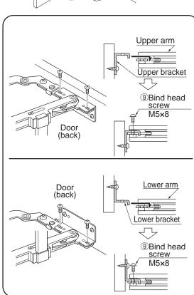
If it is difficult to screw the upper fittings from above, screw the fittings from below.
