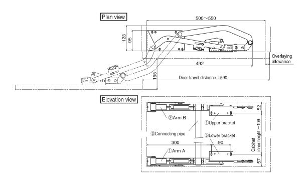
**INSTALLATION PROCEDURE** This describes the installation of a left-handed door.
