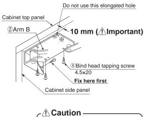
Be sure to fasten the screws firmly to prevent the bracket from coming
