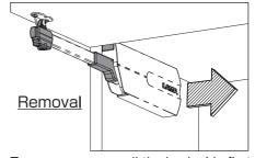
To remove cover, pull the back side first.
