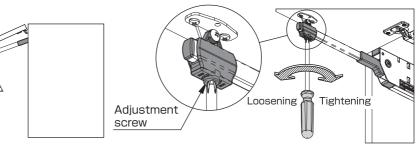
·If you feel that the door is too light (self lift-up) or too heavy (self-closing), it is possible to limit the action of the spring by tightening the adjustment screw.
