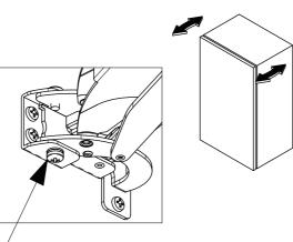
Leveling ajustment screw Back
