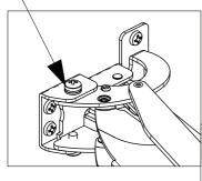
Loosen both screws, adjust the door and retighten screws.
