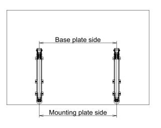
Ensure that the two LIN-X bodies are parellel by measuring both the base and mounting plate distances.
