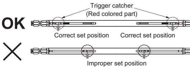
If the trigger position is wrong, pull back the trigger catcher to the correct position using a 6 mm diameter round bar.
