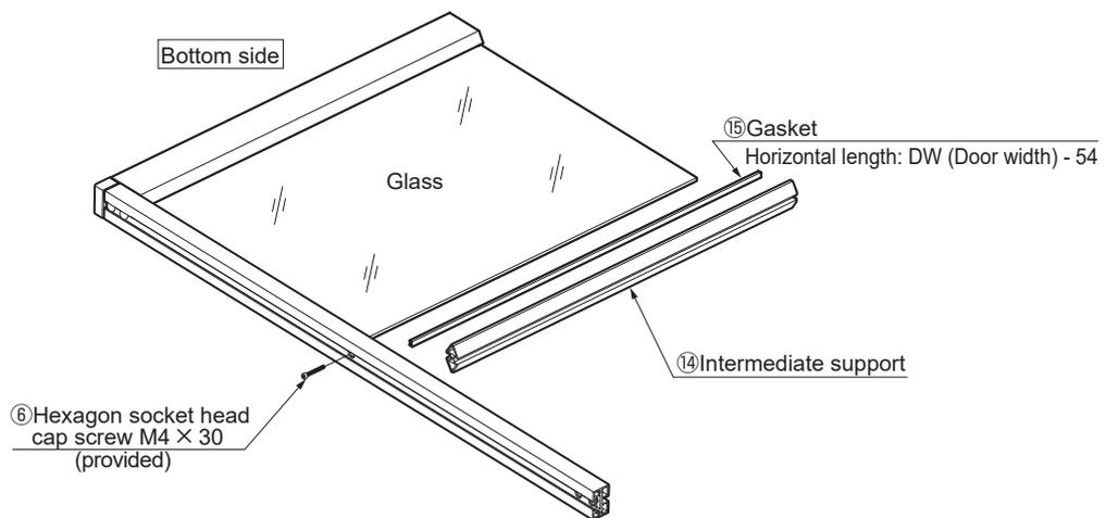
**[5] Insertion of glass - Step 2, when Intermediate support is used.**
