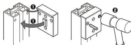
① Hook the jig on the upper edge of the vertical frame and the groove.
