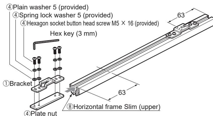
Fasten the bracket to upper horizontal frame ⑦,⑧, using plate nut ④.
