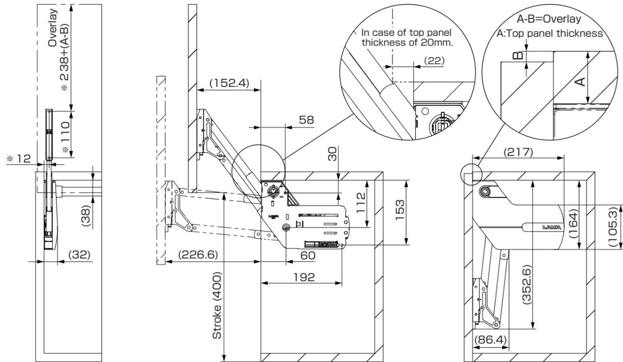
· In case of inline top & bottom doors, make sure to leave a gap of more than 3mm (if door thickness is 16 ~ 22mm).
