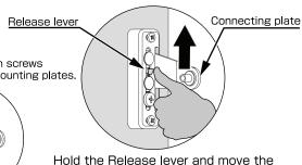
Hold the Release lever and move the connecting plate up until it stops.
