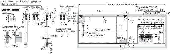
dimensions in [ ]: When recessed guide track (option) is used. ( ): When long shaft floor guide (option) is used.
