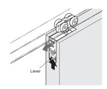
4. Adjusting Floor guide: adjust range is ±2 mm. Slowly close and open the door. If door is not moved smoothly, it is necessary to make forwardbackward adjustment for floor guide and door.
