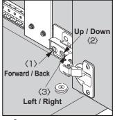
·Do not use motor screwdrivers. ·Be careful not to overtighten the screws.
