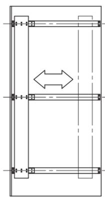
(1) Hold the Connecting plate and move it from the front end to rear end, and align the Rails so that the Connecting plate moves smoothly.
