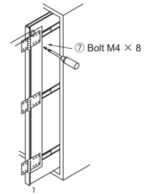
Mount the door to the Connecting plate on the Middle board. Ensure all of the screws are tightened firmly.
