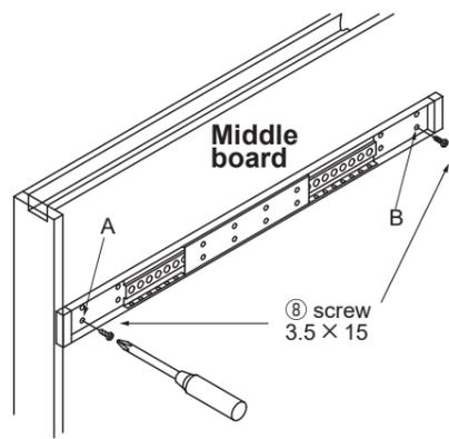
Mount rails by hole A and B temporary.
