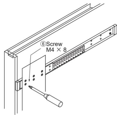
Mount Connecting Panel to the rails by 6 screws each. Check if all screws are tightened firmly.
