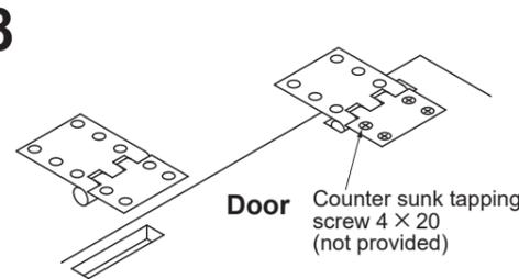
Mount Hinges to the specified positions (see the drawing of "Door processing"). The position must be correct since the hinge is not adjustable.
