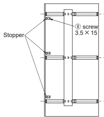
Mount Stoppers to the specified positions (see the drawing of "Side view").
