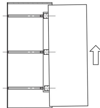
When the door is inclined like Figure 1, loosen the bolts and counter sunk screws on the hinges. Hold the door to the opposite inclination like Figure 2, then re-tighten the screws and bolts.
