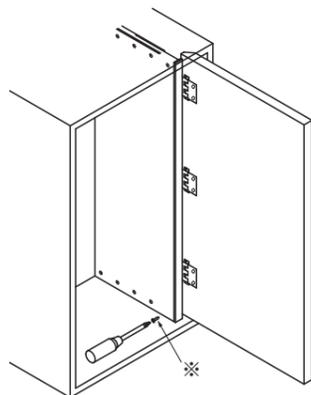
Insert the Middle board fully, and fix it. Check if the Middle board is straight before fixing.
