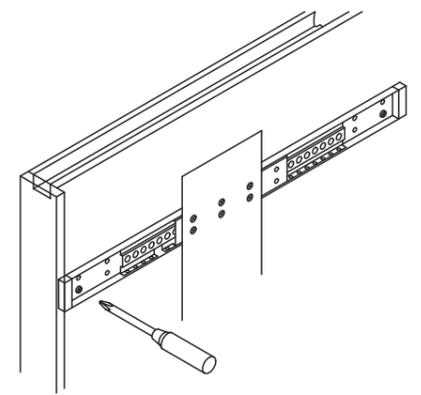
Fix the rails by screwing all of the accessible holes. Ensure all of the screws are tightened firmly.
