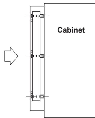
Insert the Middle board in the cabinet, but leave some part for the mounting of door.
