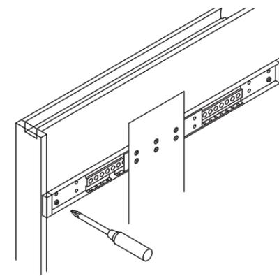
If the movement is OK, tighten the two screws firmly and check the movement again. If the movement is not smooth, do it again from procedure 3. Proceed to procedure 5.
