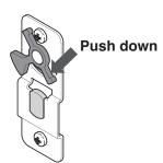
**4.**Rotate both lock pieces to the detent position.
