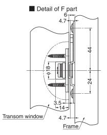
1. Mount ① Bracket to the frame, ② Hinge to the transom window.
