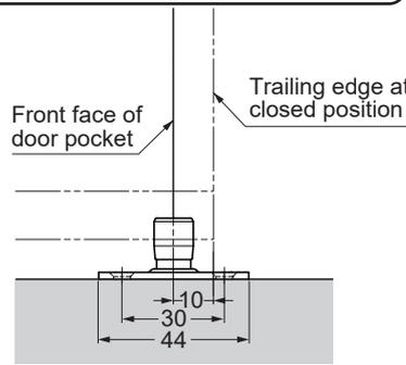
Temporarily fasten through the slotted holes with the provided screws.
