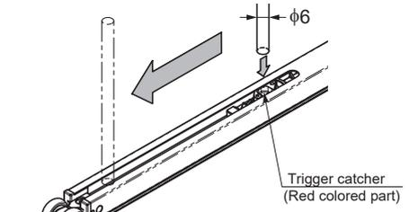
If the trigger position is wrong, pull back the trigger catcher to the correct position using a 6 mm diameter hard bar.
