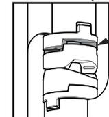
Check the hinge assembly before hanging the door. If there is a gap in the bush assembly, please turn the bush 180° and ensure that there is no more gap.
