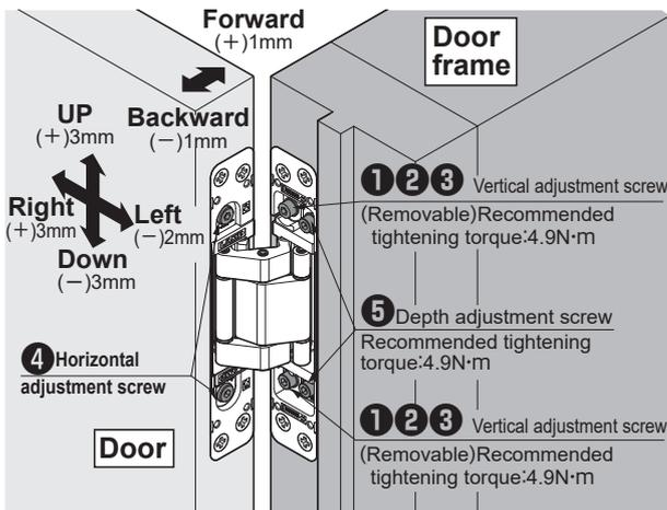
①—⑤ is the order of adjustment. Please put a supporting spacer under the door when adjusting it. There are two adjustment screws on one hinge.
