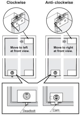
For doors with a cam lock,, check the movement of the deadbolt or cam when adjusting door position.
