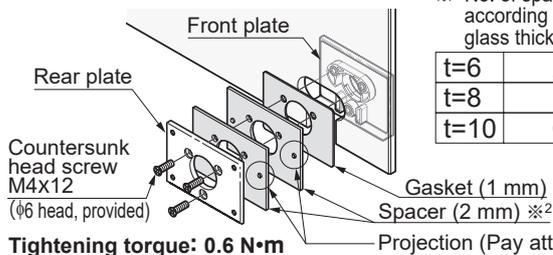
※<sup>2</sup> No. of spacers according to the glass thickness
