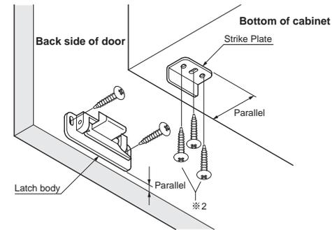
**STEP-3** Check how the latch works by opening and closing the door.
