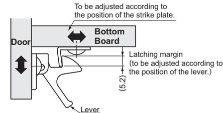
In the case that the door joints were adjusted at the hinges, adjust the latch accordingly.
