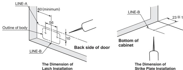
**STEP-2** Mount the body of the unit to the back of the cabinet door and mount the strike plate to the bottom of the cabinet, but do not tighten the screws down at this time.
