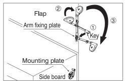
Turn the main body 90 degrees (2)and insert the pin of the mounting plate in the hole of the main body.
