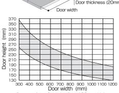
\*In case of usual wooden flap of 20mm thickness (specific gravity approx. 0.5)
