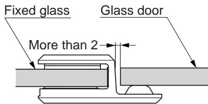
⚠ Clearance between the stopper and door must be more than 2mm.
