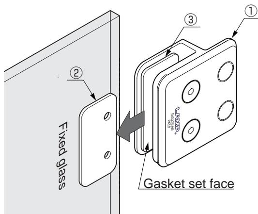
3 .Tighten attached screws to tighten the stopper ① . Recommended torque: 1.5 N/m
