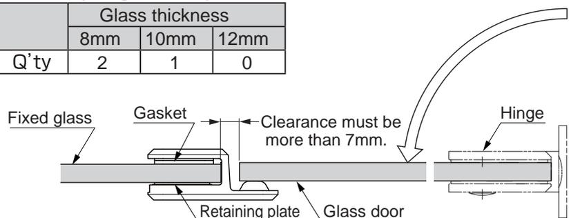
2 .On the gasket set face, paste required quantity gasket ③ . And, install stopper ① .
