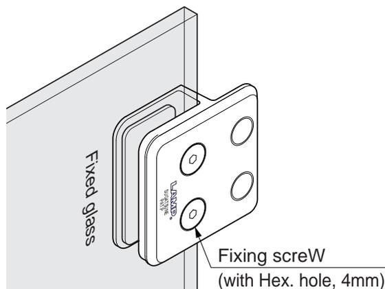
**■ In order to reduce the clearance between door and fixed glass with glass cutout.**
