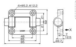
✓!\Screws not included Recommended screw and washer M5 hexagon socket head screw × 4 washer 5mm in nominal diameter × 4
