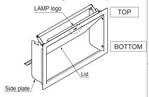
Do not leave any gap between the flap lid body and the mounting surface.
