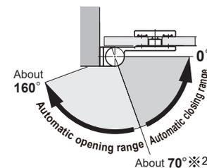
※2 The maximum lifting of the door is 3 mm when the opening angle is 70°.
