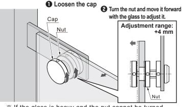
\* If the glass is heavy and the nut cannot be turned, lift the glass slightly.
