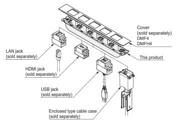
[2] Starting from either end, hook the jack onto the lip of the bracket and push until a click sound is heard.
