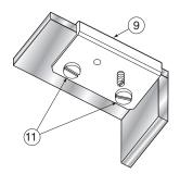
Set fixing screws 11 into top plate glass hinge support 9, and tighten them using a flat head screwdriver.
