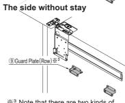
¾³ Note that there are two kinds of guard plates (high) and (Low). If the guard plates are not enough to avoid interference with stored articles, install a middle plate.
