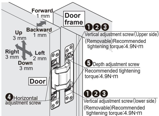
①—⑤ is the order of adjustment. Please put a supporting spacer under the door when adjusting it. There are two adjustment screws on one hinge.
