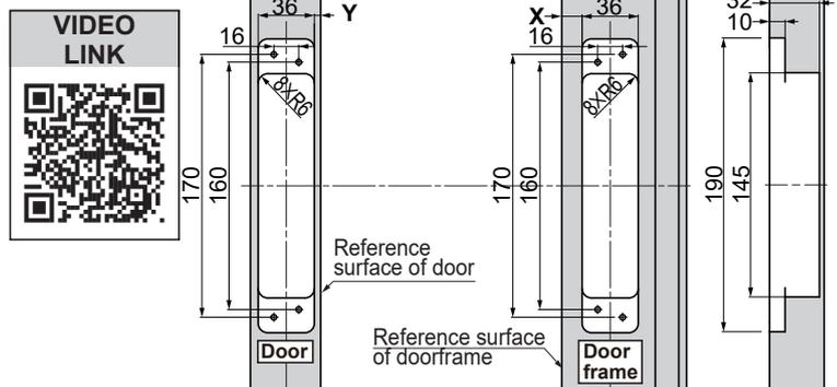
When not using the installation template HES3D-W190-TMP (sold separately) drill pilot holes at the installation screw locations.
