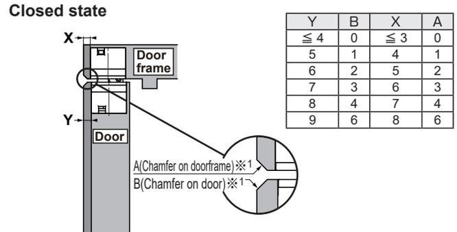
※ 1 Chamfer is needed depending on the amount of X and Y.
