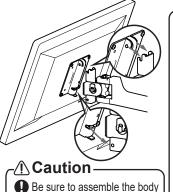
and the mounting plate from the same package delivered. Make sure that the release lever is at the locked position. If not, the mounting plate may be disconnected when the monitor is moved. Release lever
