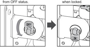
Above drawings show tilt lock. The way of swivel lock is the same.
