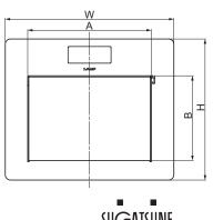
AZ-AT230-HL 4×R6 Max. \_147.5 Mounting screw holes 142 132.5 +0.5 153.2 +0.5 Cut out: Backside view
