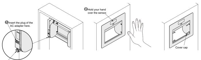
Adjust the sensing distance with this knob Clockwise: Increase up to 300 mm Anti-clockwise: Decrease to 0 mm (No sensing) 4 Use the wiring clips so that the wire does not interfere with the contents of the waste container. Recommended screw: Pan head tapping screw \$3
