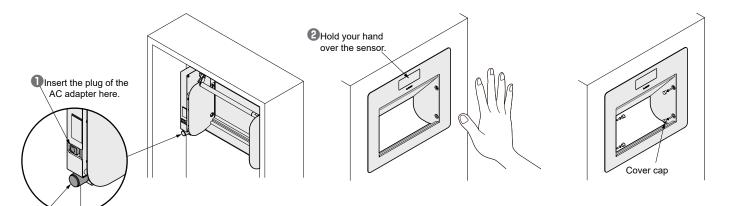
Adjust the sensing distance with this knob Clockwise: Increase up to 300 mm Anti-clockwise: Decrease to 0 mm (No sensing)
