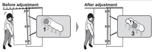
**3 Tighten all** the temporarily fastened screws
