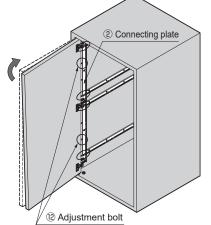
3 Tighten all the screws once the door is in the desired position.
