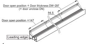
Trigger mount hole must be done, taking care direction of door (door head side and door tail side)
