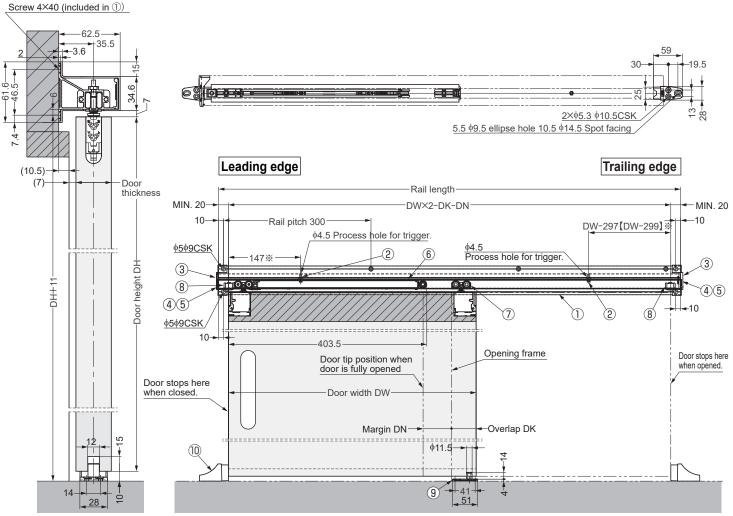
% If the left and right sides of the door are opposite to this picture, please reverse the trigger mounting hole from side to side.
