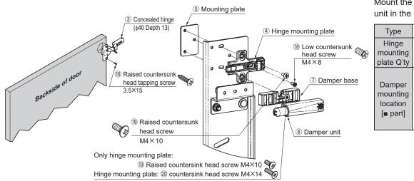
Mount the damper base and damper unit in the specified position.
