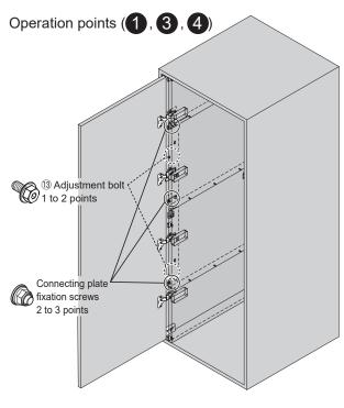
2 Lift the door and shift the adjustment bolt backward one level at a time, to make the door and connecting plate vertical.
