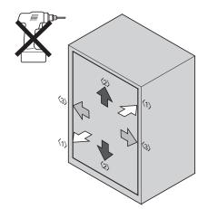
Carry out the adjustment from the hinge access hole with the door opened
