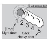
When there are adjustment bolts at top and bottom, align their positions.
