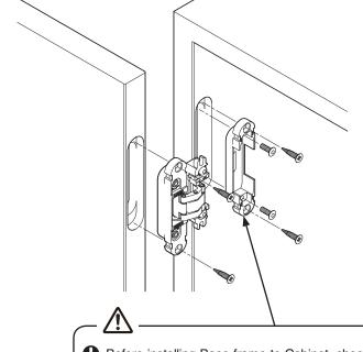
Before installing Base frame to Cabinet, check the mounting direction by coupling it with Hinge main body.
